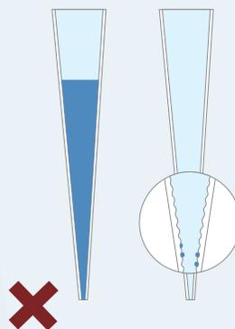
A rough inner wall will hang up liquid in a tip, resulting in poor accuracy/precision.
