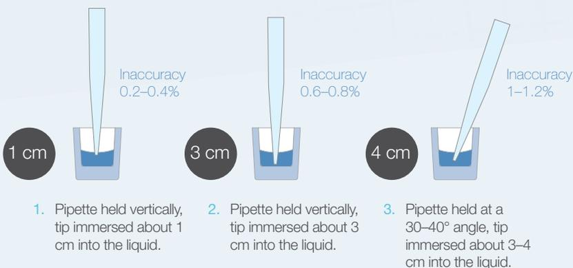
**Step 1:** The tip is immersed to the correct depth and correctly held vertically.
