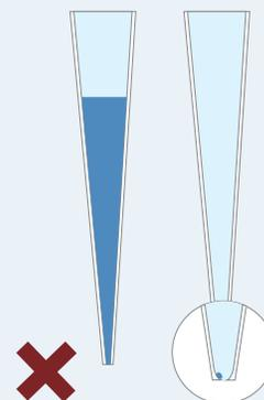
Flash at the orifice can hang up liquid, resulting in poor accuracy/precision.
