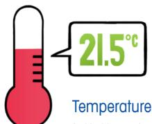
An ideal temperature for pipetting is 21.5°C (±1°C). Your instrument and samples should be the same temperature as the room in which you're working, so allow them to equilibrate for 20 minutes if necessary. Also avoid drafty or sunlit areas that can cause large or sudden temperature changes. Pipetting at a constant temperature improves results by as much as 5%.
